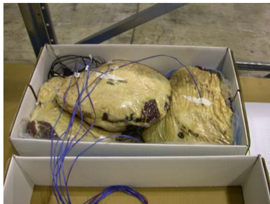
Fig 13: Vacuum packaged rumps showing placement of thermocouples and contact areas
