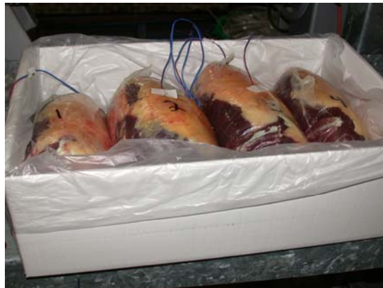
Fig 12: Individually wrapped rumps showing placement of thermocouples and contact areas
